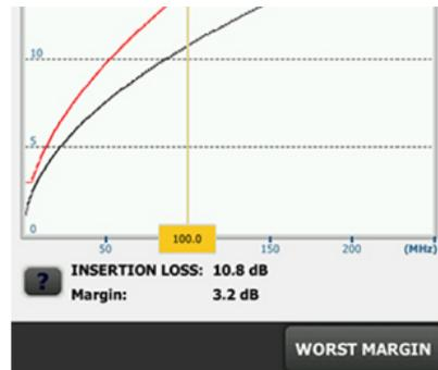
Figure 2. Measured Insertion Loss and limit for 450 foot Type 734 cable.
