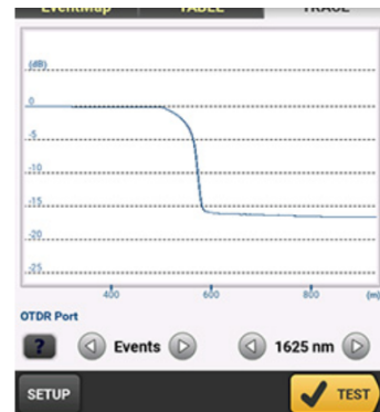
Splitter as seen on an OTDR trace
