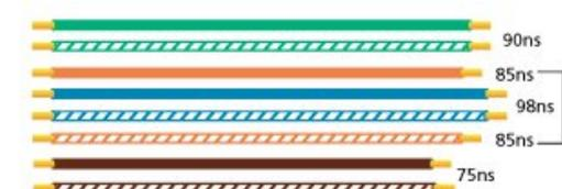
Longest delay = 98 ns, shortest delay = 75 ns. Delay skew is 23 ns.
